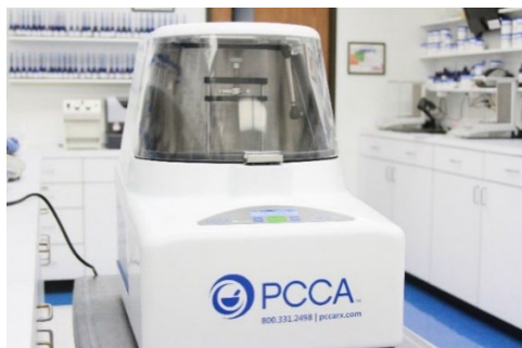
Figure 1. PCCA RAM™: ResonantAcoustic® Mixer.
